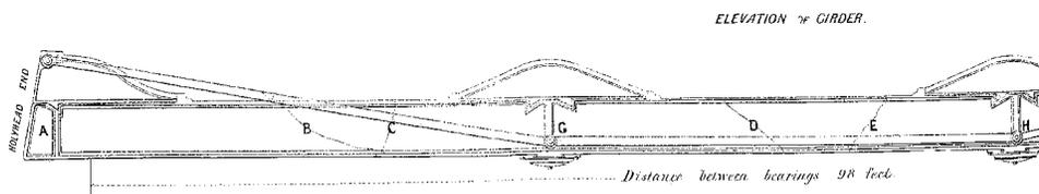
3 Section of broken girder from accident site showing two main fracture zones, BC on the casting nearest the Holyhead end of the girder and DE on the centre casting (from Simmons' report)
